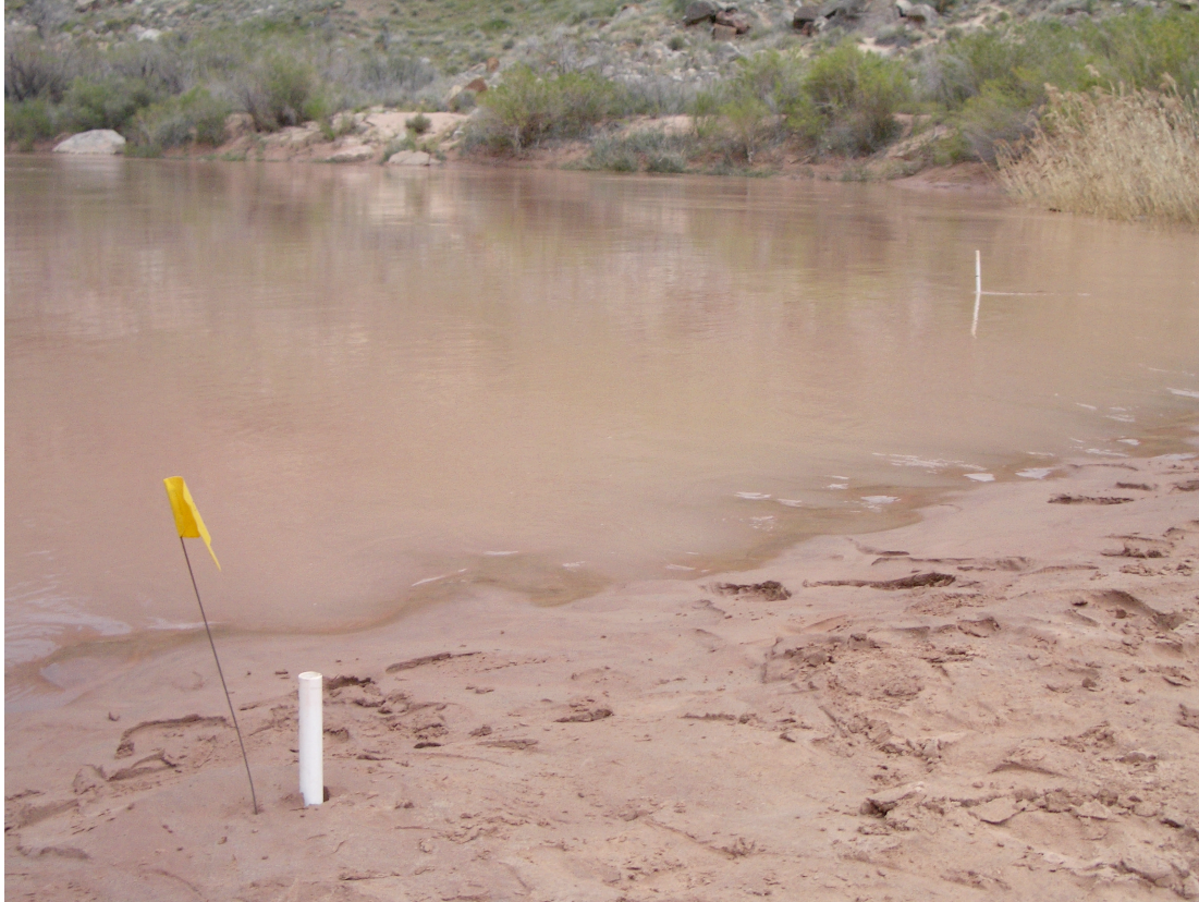
Figure 2. Setup of experiment to measure river stage and sandbar stage fluctuations during drawdown.
