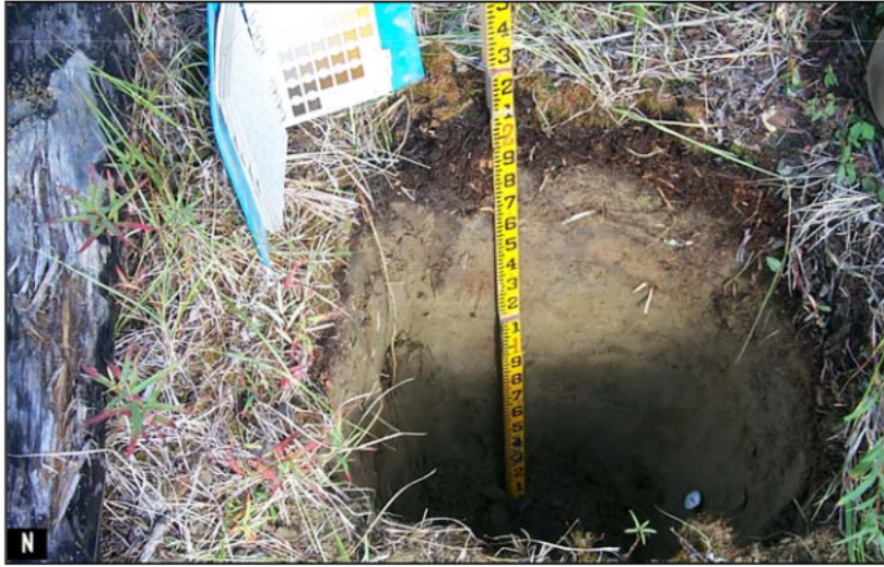
Figure 8. The effects of fire on a soil profile. This profile was highly organic, with gleyed subsurface, indicating very wet conditions. After a fire, much of the organic mat was removed, the permafrost melted, and the soil now resembles the warmer drier soil shown in Figure 7. Photo courtesy Mark C. Rains.
